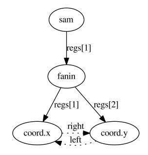
The frontend sets up the SSA ptrs from sam source register to the fanin meta instruction, which in turn points to the instructions producing the coord.x and coord.y values. And the grouping pass sets up the left and right neighbor pointers to the fanin's sources, used later by the register assignment pass to assign blocks of scalar registers.
