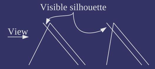
Amount to bias back-face depends on both slope of back-face and slope of front-face
