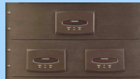
Shown here is a single PIMM in a 1-PIMM Garage racked on top of two PIMMs mounted in a 2-PIMM Garage
